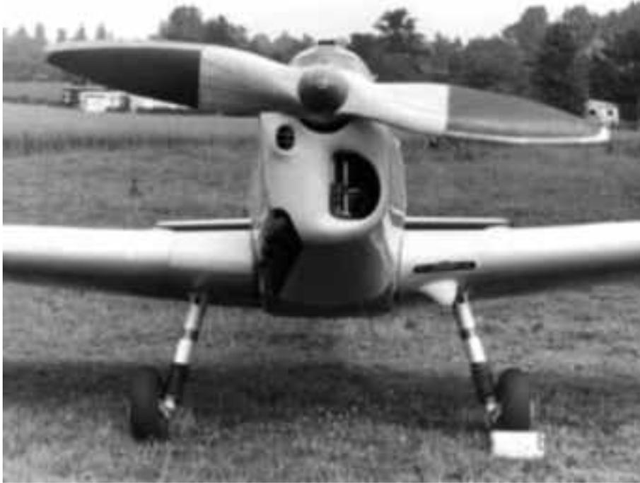
steerable tailwheel doing most of the work. Take-off acceleration was rapid, with 160 horses pulling 818kg (1800lbs) quickly into the air. Following an unstick at about 85km/hr (53mph) the Zlin of the time was soon at the recommended climb speed of 120 (75) with a surprisingly nose-up angle producing a very creditable 1350 feet per minute.
